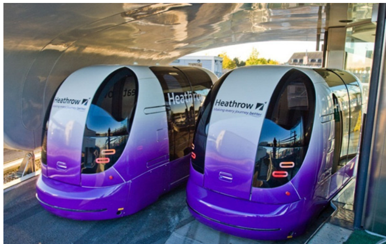
Heathrow PRT four-seater battery-electric vehicles
