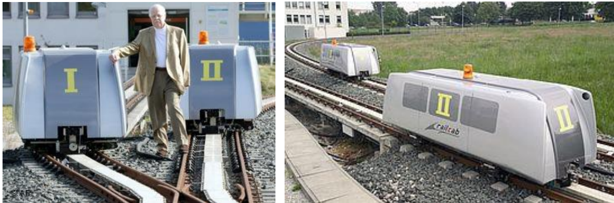
Figure 2.2a & 2.2b: The RailCab project test segment in Paderborn, focussing on rail DRT vehicle technology.
